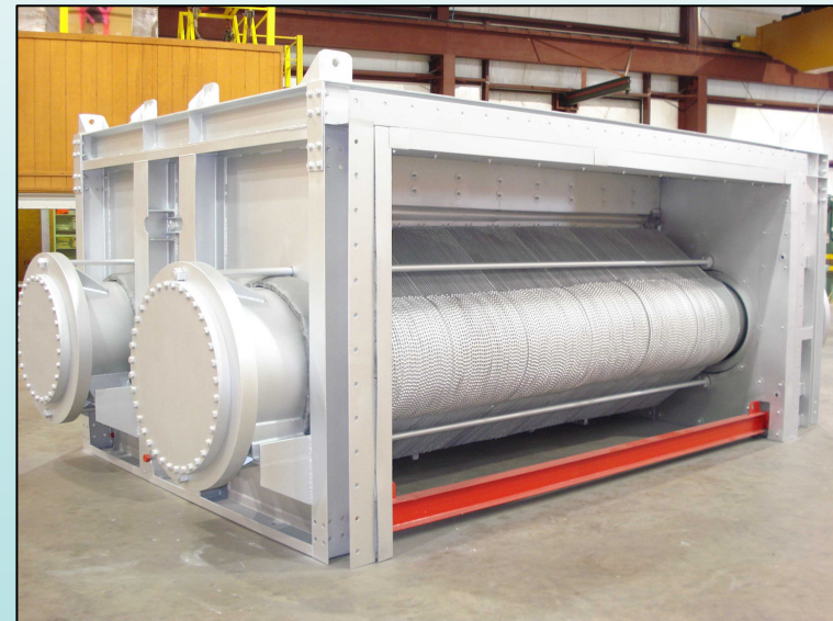
Gas Turbine Regenerator
